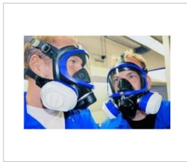
**Combined protection** – may incorporate eye protection. There are a number of designs that integrate head, eye and respiratory protective in one unit. The eye protection can stop projectiles and chemicals from entering and injuring the wearer's eyes and provides head protection at the same time, in addition to respiratory protection, usually by supplying the wearer with filtered air or air via a compressed air line.
