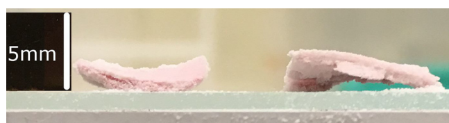
Fig. 6. Warping of 3D printed 9:1 cellulose LBG powder.
