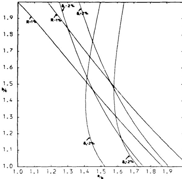
Fig. 3. Plots of the contours of constant value for the functions  $R$ ,  $\delta_+$ , and  $\delta_-$  at  $\pm 1\%$  levels. Other details as in Fig. 1.
