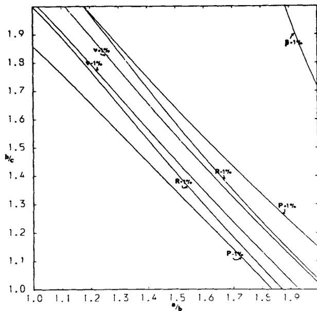
Fig. 2. Plots of the contours of constant value for the functions  $\nu, P, \beta,$  and  $R$  at  $\pm 1\%$  levels to simulate error in measured values. Other details as in Fig. 1.
