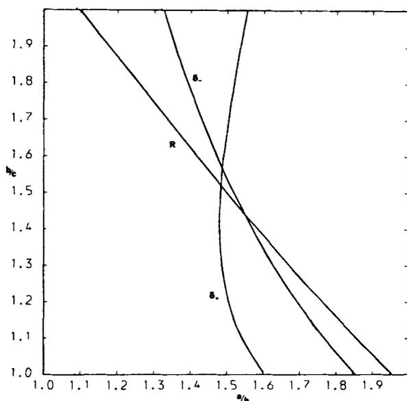
Fig. 4. Plots of the contours of constant value for the functions  $R$ ,  $\delta_+$ , and  $\delta_-$  (as in Fig. 3) assuming no error greater than computer rounding error in supplied data. The nonlinear least-squares method (see text) was used.
