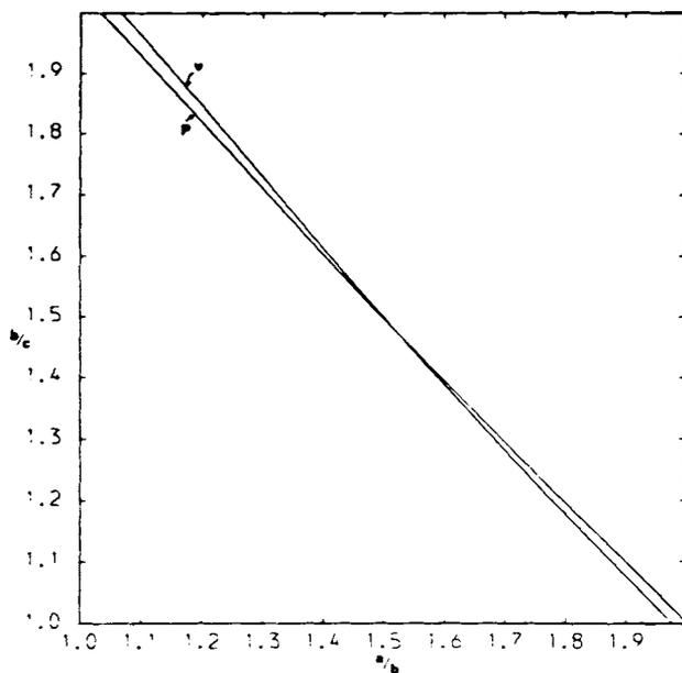
Fig. 1. Plots of the contours of constant value for the functions  $\nu$  and  $P$  in the  $(a/b, b/c)$  plane, computed for the values  $a/b = 1.5, b/c = 1.5$  for the two axial ratios of a tri-axial ellipsoid.
