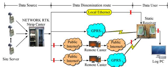
Fig. 7. Experimental plan for evaluating correction delay and loss (Ntrip: a dedicated protocol for transmitting geodetic data over the Internet).
