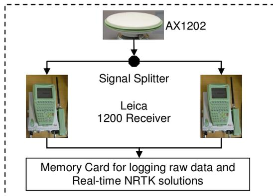
Fig. 3. A configuration for roadway data acquisition.
