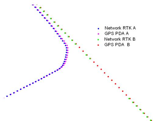
Fig. 8. Comparison of the trajectories generated by a geodetic GNSS receiver and cheap HSGPS receiver
