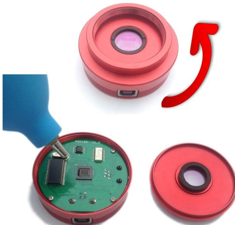
The sensor is an optical device. All precautions must be taken to prevent dust or scratches on the input window. If there is dirt that doesn't come off with the air pump, here is the step to clean it.
